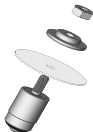
Drawing 2: differential valve replacement kit – piston assembly (35006090)
